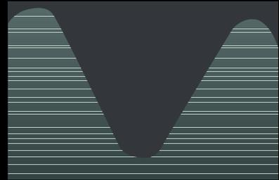
Metal flows refer to the flows of the metallographic structure. Precision cold forging, which does not involve machining the gear tooth surfaces, does not interrupt the metal flows. The gear, with its metal structure preserved along the processed shape, is highly resistant to impact and exceptionally difficult to break.
