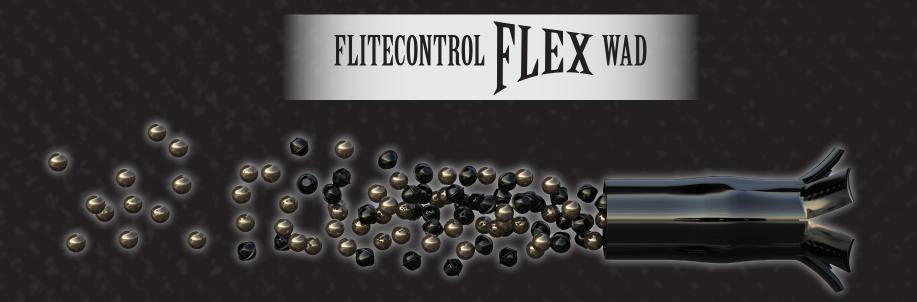
The FLITECONTROL FLEX<sup>®</sup> wad opens at the rear, creating an air brake that pulls the wad off the shot string. The pellets are released at the optimum moment for accuracy and power. The wad is combined with unique shot types to get better performance on target.
